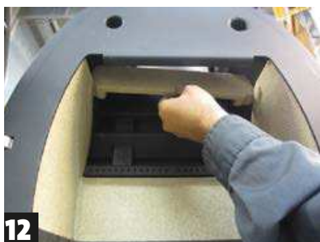
12 Lift the plate over the side plates
