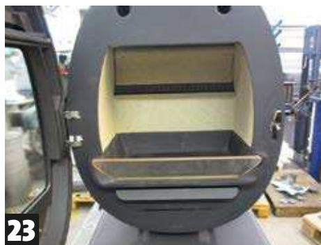
20 Push the plate backwards in order to mount the pins
