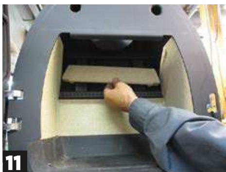
11 Pass the plate towards the rear
