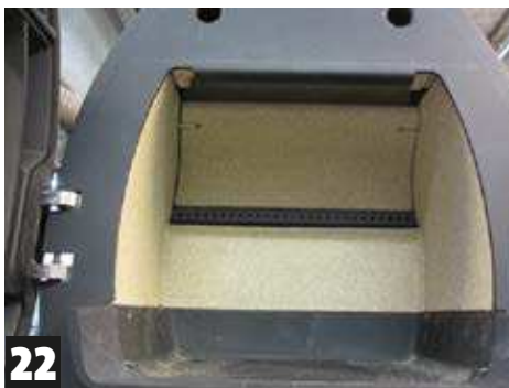
19 Let the plate rest on the rail with the air slots
